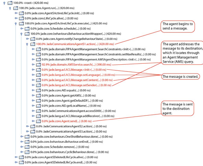
Fig. 16. Dynamic analysis data for Jade static agents. Here, the agent is initialized and run by the framework.
