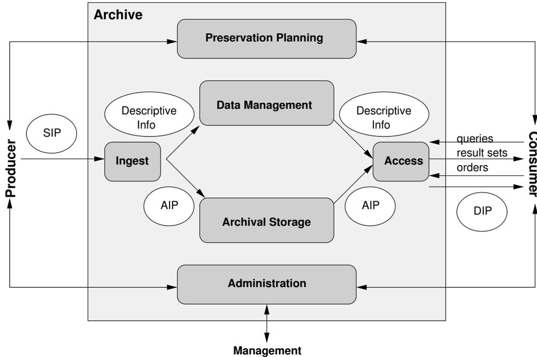
Figure 2. OVERVIEW OF FUNCTIONAL COMPONENTS AND INFORMATION FLOWS WITHIN THE OAIS MODEL.
