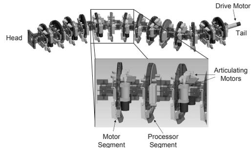
(b) A 3D CAD model of the snake robot.
