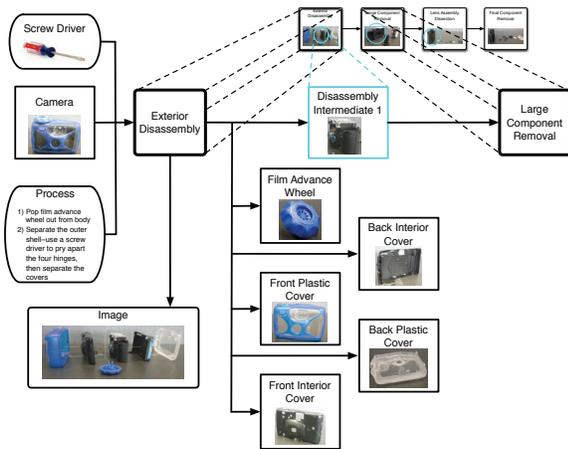
Figure 5: Product disassembly workflow for the camera.
